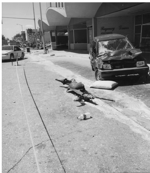
Axle from the bomb truck at Oklahoma City, located about 200 yards from the crater
